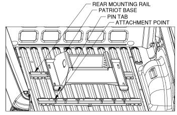
Figure C1: View into truck bed looking towards tailgate.
